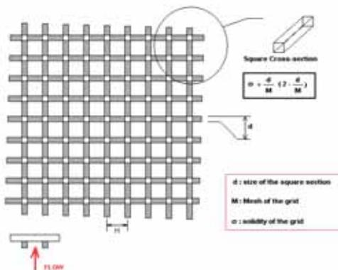
Fig. 6: Turbulence grid shape
