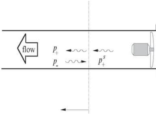
Fig. 1: An in-duct source modelled as an acoustic one-port
