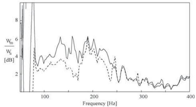
Fig. 3: Maximum emitted sound power on the outlet (a) side normalized using the sound power emitted with an anechoic load, calculated from 1-port source data measured on an axial flow fan. —, 1430 rpm; - - - - - , 2850 rpm. [10]
