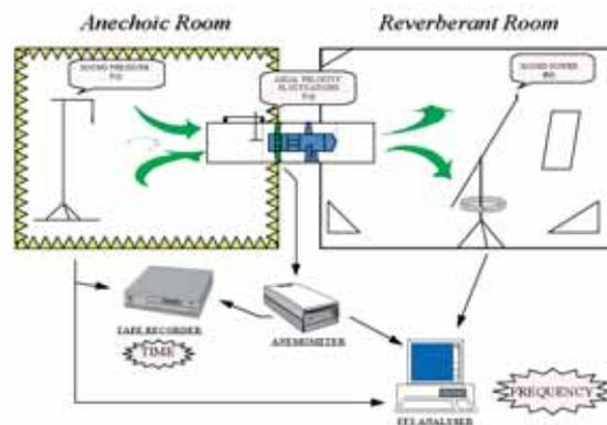
Fig. 4: e Setup used for the aerodynamic and acoustic measurements
