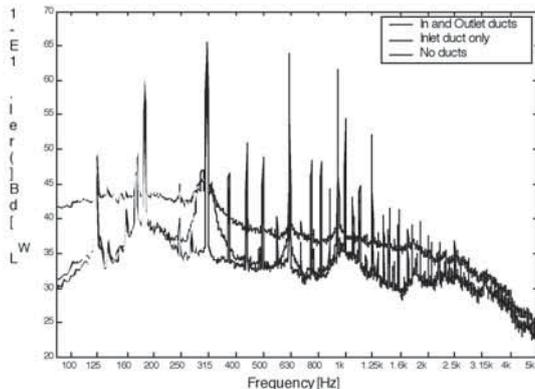
Fig. 10 : Example of sound power levels of an axial fan of mixed flow type with and without acoustically transparent ducts attached. The flow rate was kept constant
