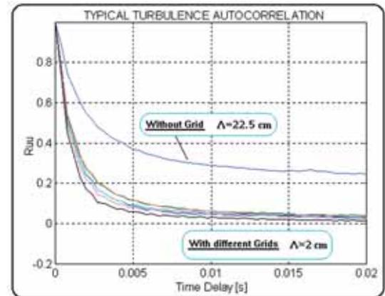
Fig. 7: Turbulence autocorrelation measurement without and with upstream mounted grids.
