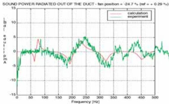
Fig. 5: Acoustic loading effect; comparison theory/experiment
