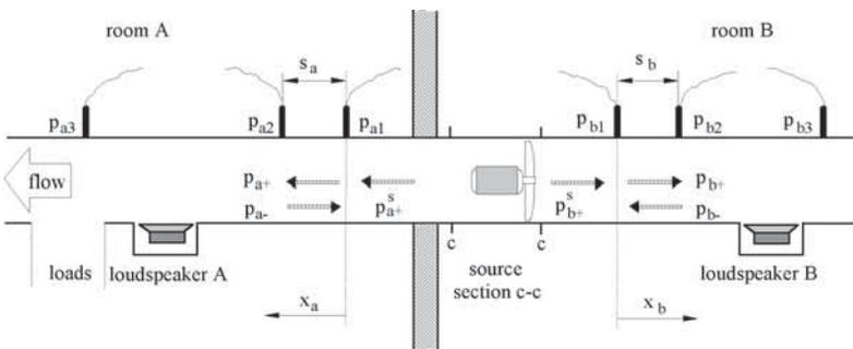
Fig. 2: Test rig for two-port source measurements.
