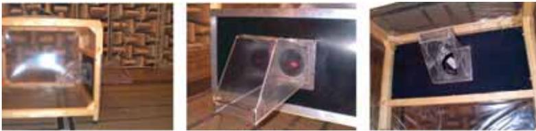
Fig. 9 : Left picture the ISO 10302 test rig with its plastic walls and a mounted fan; middle picture, duct section connected to the fan inlet; right picture, duct section connected to fan outlet. The ducts are similar to sections in a cooling fan installation for a cabinet with electronic equipment
