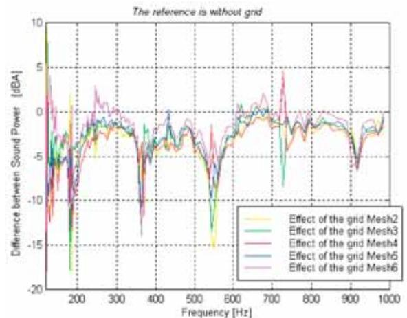
Fig. 8: Difference in fan sound power level without and with turbulence grids for 5 different grids
