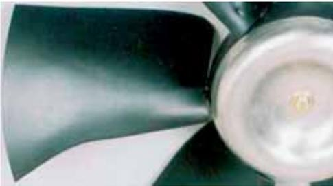
Fig. 3 : Chord length near the tip
