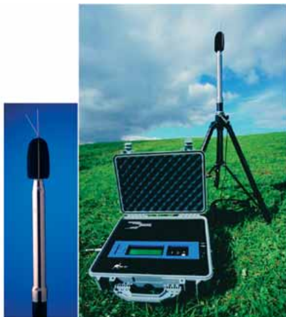
Fig. 3 and 4 : Presentation of the noise monitoring terminal (microphone and the portable unit)
