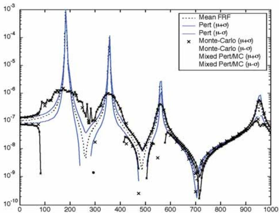
Fig. 2 : Dispersion of the vertical displacement FRF for a plate with random flatness default
