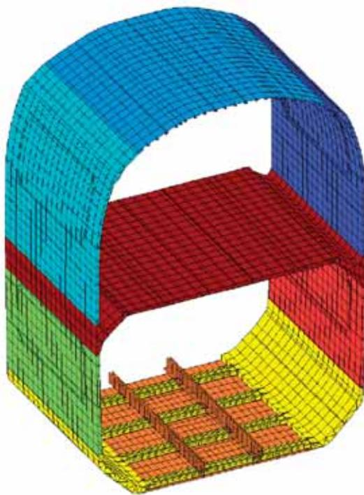
Fig 4 : Optimal SEA subsystems for a train structure model
