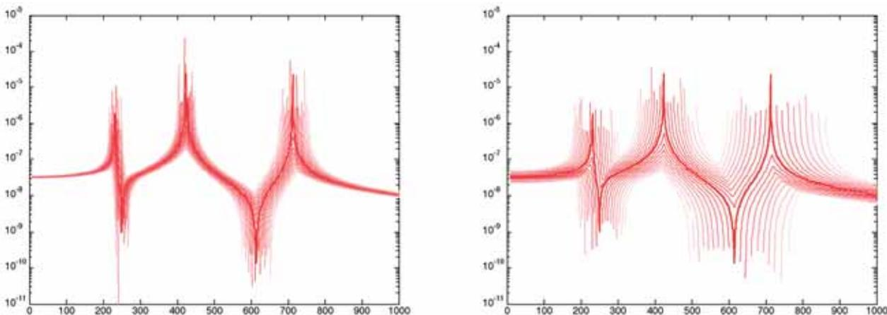
Fig. 3 : Articulated truss structure : fuzzy FRF of the displacement field (all parameters having 3% (left) or 10% (right) of variability)
