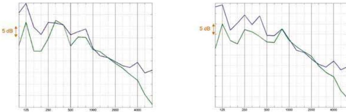
Fig.6 : SPL[dB(A)] recomposition VASM versus measurement, 4th gear 100km/h
