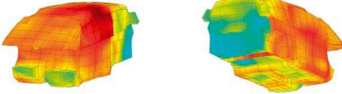
Fig. 5 : Transfer function 3DF map at 1 000 Hz, driver's position
