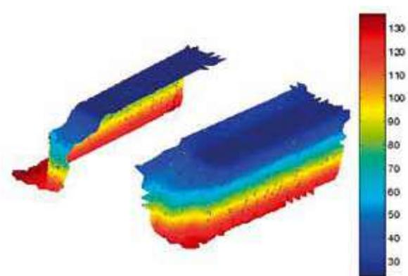
Fig. 9 : Tunnel insulator thickness cartography example
