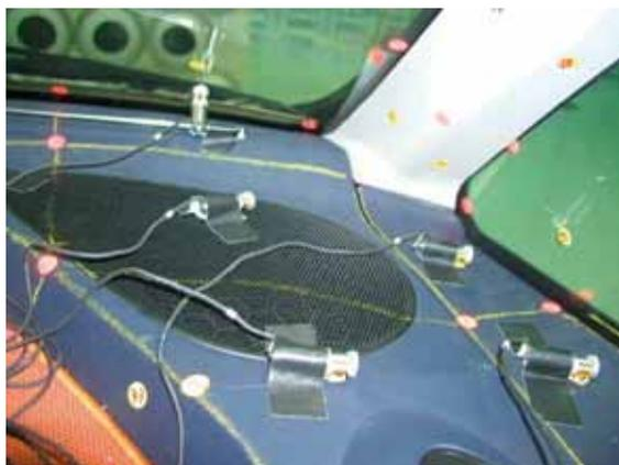
Fig. 2 : Sound power measurement protocol
