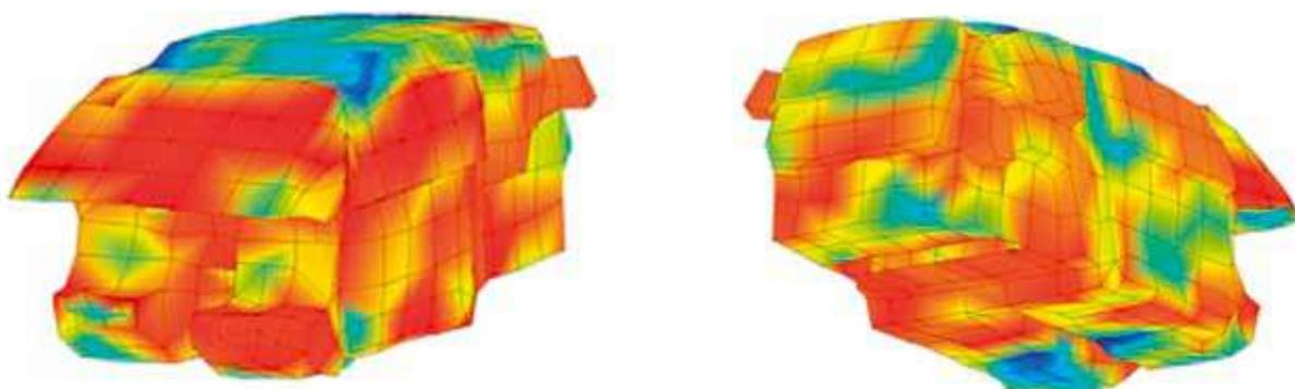
Fig. 8 : SPL recomposition 3D ma pat 1 000 Hz, 4th gear 100 km/h ; driver's position
