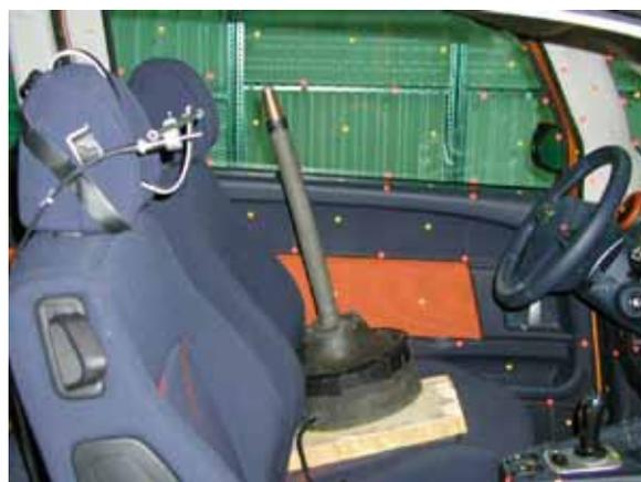
Fig. 4 : Transfer function measurement protocol
