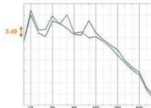
**Fig. 18 : SPL [dB(A)] measurement comparison serial optimized, 4th gear 100 km/h**
