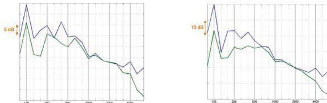
Fig. 7 : SPL[dB(A)] recomposition VASM versus measurement, 2nd gear 100km/h
