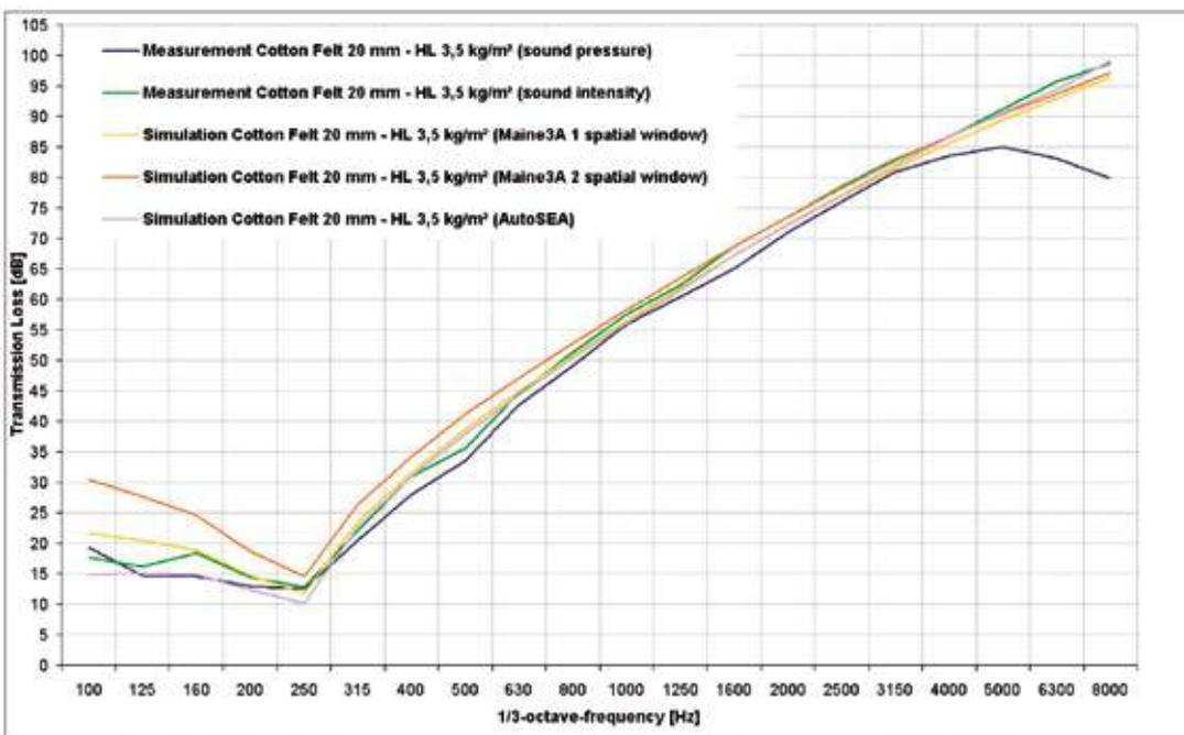
Fig. 16 : Transmission Loss : measurement versus simulation
