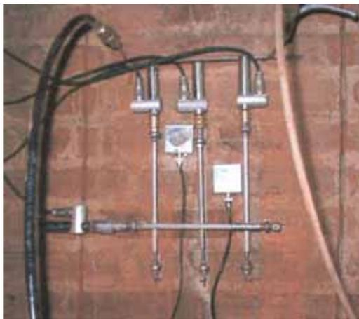
Fig. 8: Combined flat-jack test and AE monitoring
