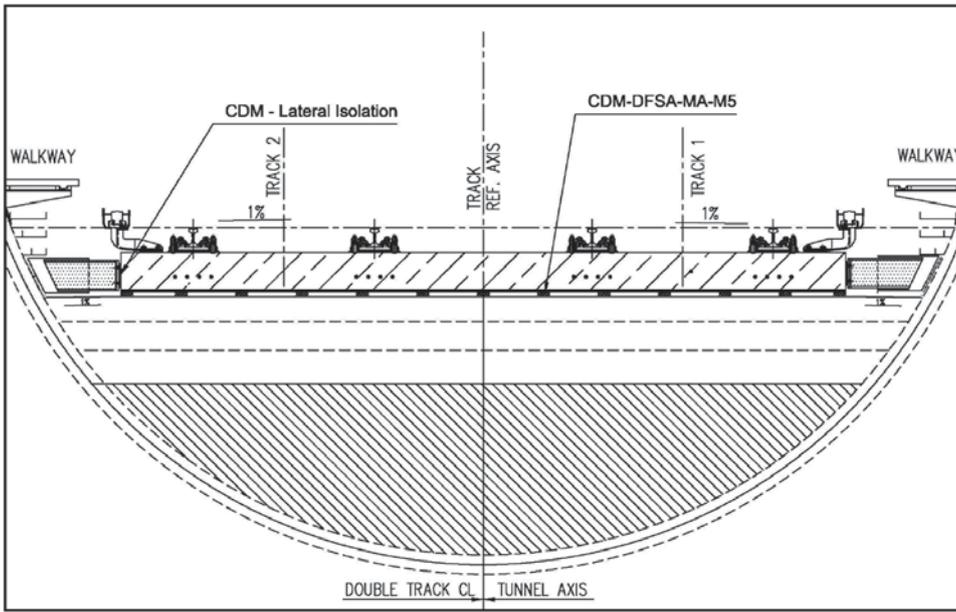
Fig. 14 : Typical construction drawing of CDM-DFSA
