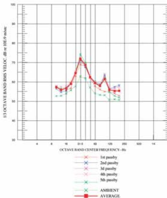
Fig. 20 : Measurements from Ethniki Amina (original twin blocks. Tangent track - building at 34 m)
