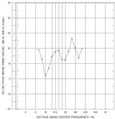
Fig. 3 : Transfer function from tunnel invert to soil surface for soil category 2 (measurement results) and for a specific tunnel depth
