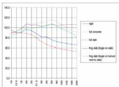
Fig. 12 : 1/3 octave band analysis for all scenarios/cases : vibration velocity spectrum for point on tunnel invert under the frog (dB ref 10-9 m/s)
