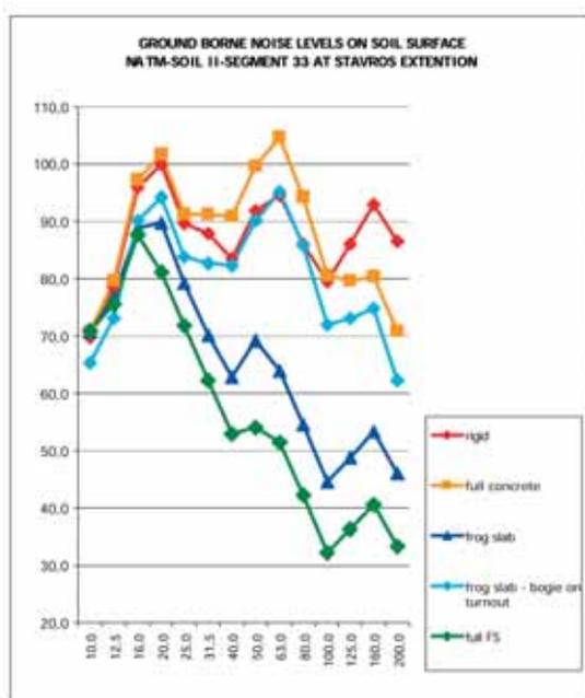
Fig. 13 : Ground borne noise levels for a typical building at the soil surface for all cases
