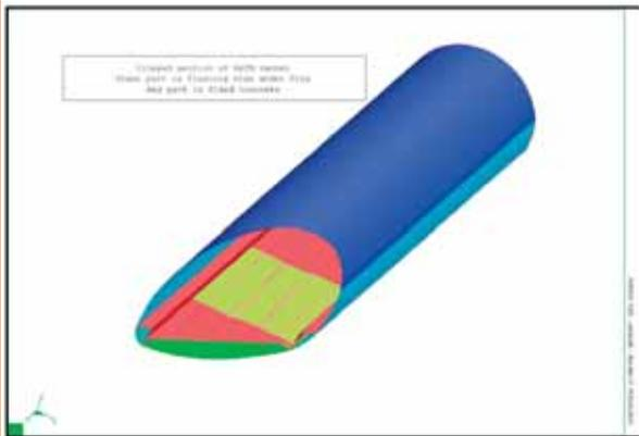
Fig. 10 : 3D geometrical model of the NATM tunnel for scenario 3
