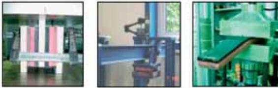
Fig. 15 : Mechanical Material Tests (in CDM-lab – k-stat, k-dyn, creep and shear modulus)
