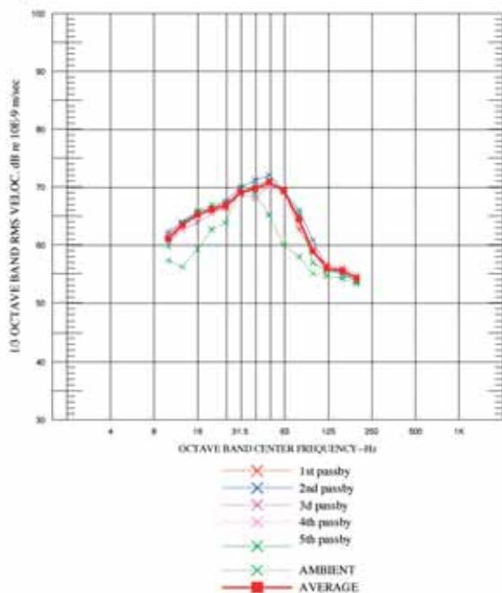
Fig. 19 : Measurements from Ethniki Amina (turnout with FST – building at 11 m. from source)
