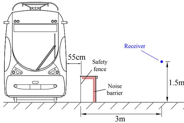
Fig. 4 : Cross sectional schematic showing relative positions of the tram, low-eight noise barrier prototype and receiver location
