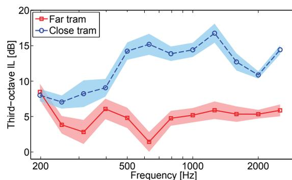
Fig. 9 : Mean values and uncertainty interval of measured third-octave insertion losses in dB in the frequency range 200-2 500 Hz. Solid line : far tram - Dashed line : close tram
