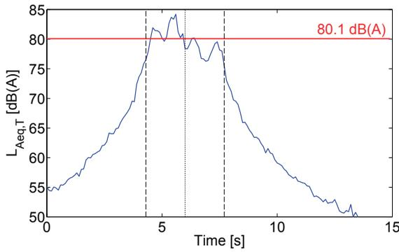
**Fig. 6 :** Example of a time history of  $L_{Aeq,T}$  in dB (A) during a tram pass-by (close tram, without barrier). The dotted line corresponds to the centre time, and the two dashed lines correspond to the initial and final instants of the pass-by. The equivalent pass-by level  $L_{Aeq,pass}$  is indicated on the plot as well
