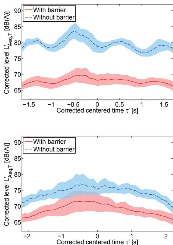
Fig. 8 : Mean and dispersion interval (plus and minus one standard deviation from the mean) of corrected levels  $L_{Aeq,T}$  time histories in dB(A) during tram pass-by as a function of corrected centered time  $\tau'$ , with (solid line) and without (dashed line) the noise barrier. Left : close tram. Right : far tram.
