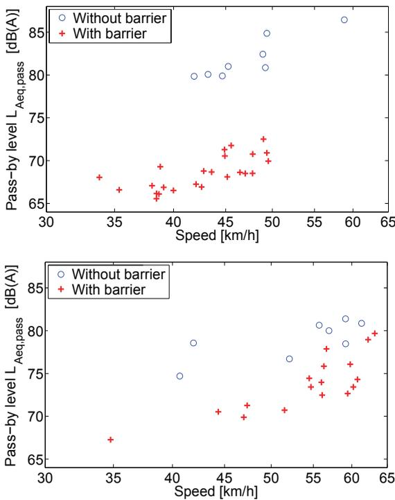
**Fig. 7 :** Tram pass-by A weighted equivalent levels  $L_{Aeq,pass}$  as a function of speed for all measurement configurations. High - close trams ; Low - far trams. Symbols : circles - without barrier ; crosses - with barriers
